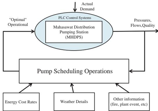
Fig. 2 MHDPS control system
