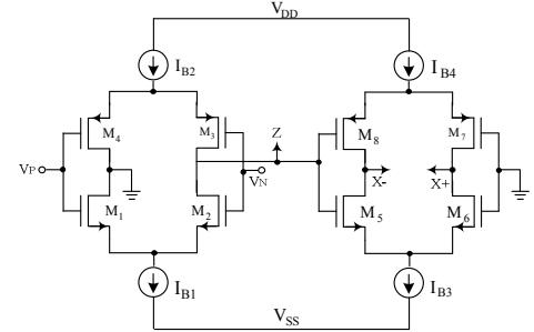
Fig. 4 Practical realization of the VDTA
