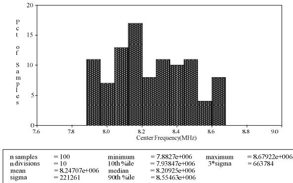
Fig. 9 Monte-Carlo statistical result of BP filter in Fig. 6 with 10% deviation in capacitor values
