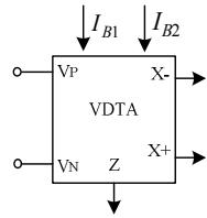
Fig. 3 Circuit symbol of the VDTA
