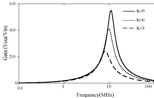
Fig. 8 Frequency responses of the second proposed shadow filter in fig. 6
