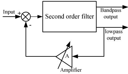
Fig. 2 The basic concept of the shadow bandpass filter
