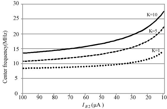
Fig. 8 Relationship of the center frequency and gains
