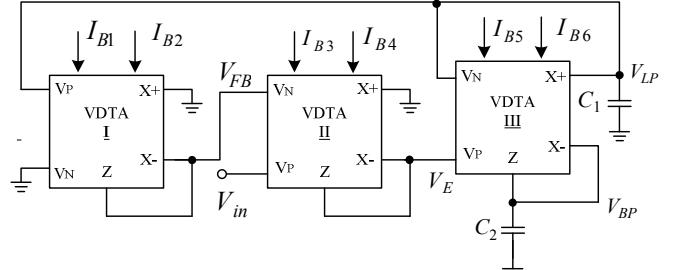
Fig. 5 The proposed shadow bandpass filter
