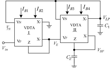
Fig.6 The second proposed shadow filter
