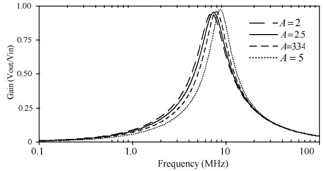
Fig. 7 Frequency responses of the proposed shadow bandpass filter in Fig. 5
