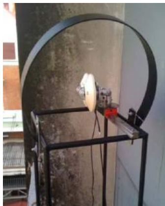
Fig. 2 The pyranometers and a shadow ring
