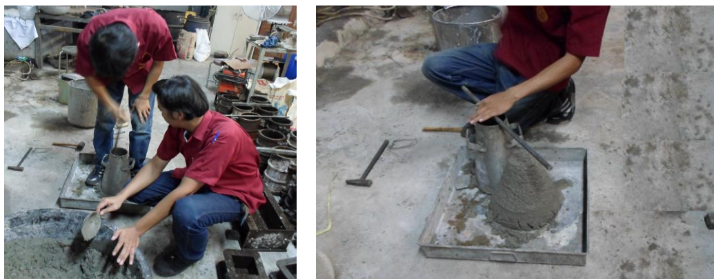
Figure 3. Slump test of concrete
