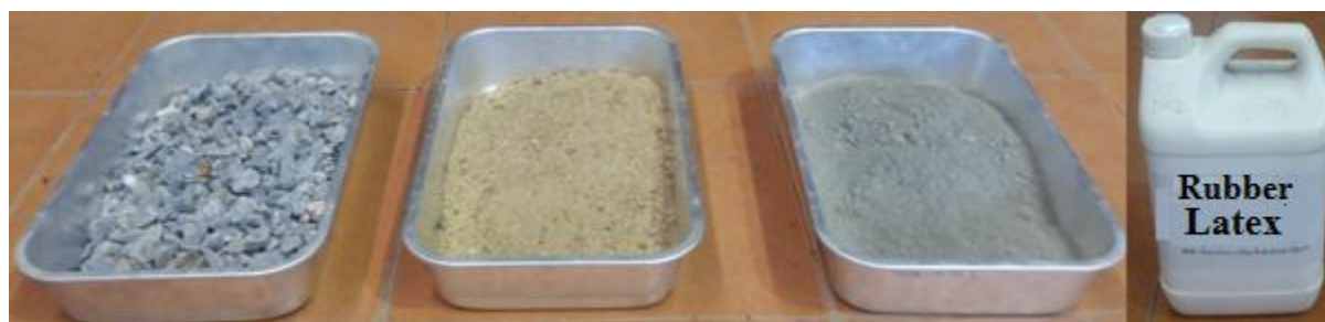
Figure 1. concrete material : Coarse aggregate, Fine aggregate, cement and rubber latex
