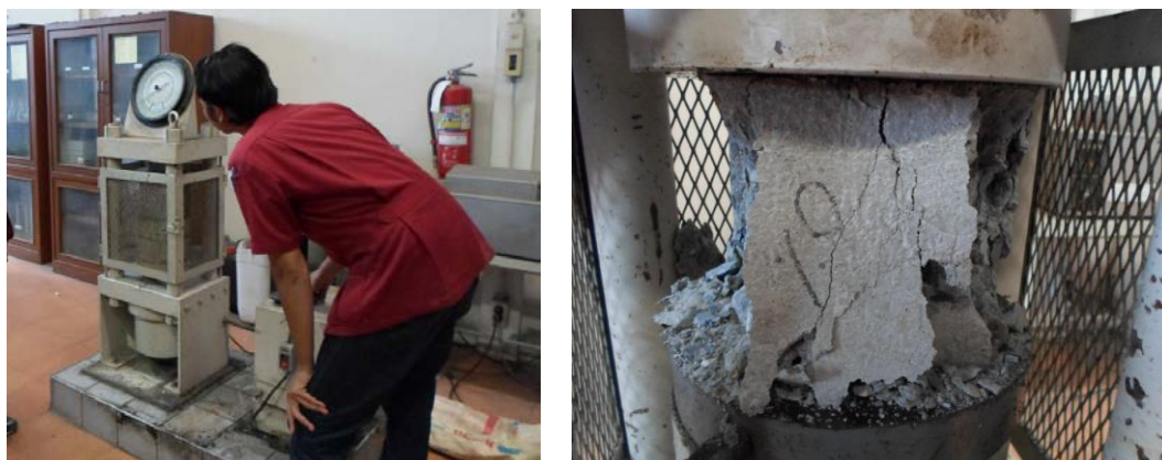
Figure 5. Cube specimen compressive strength test
