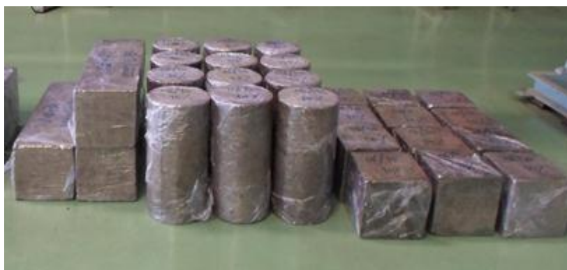
Figure 2. Curing of specimen
