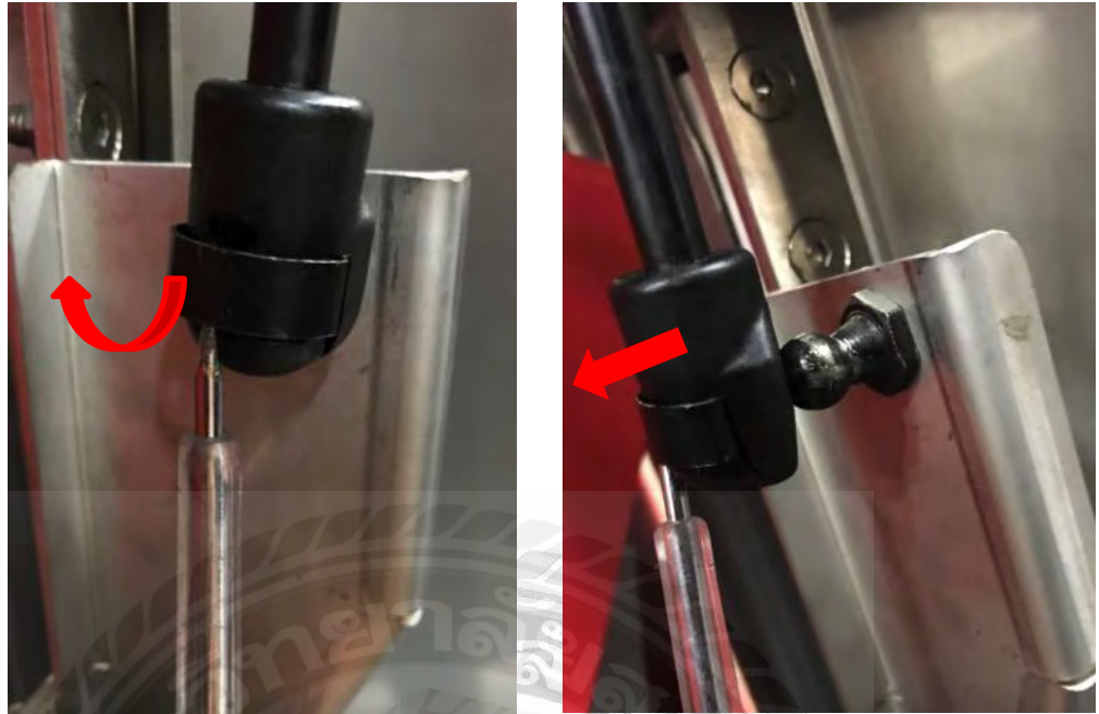
Figure 5-45 Method of Disconnecting the Gas Spring from the Ball Joint
