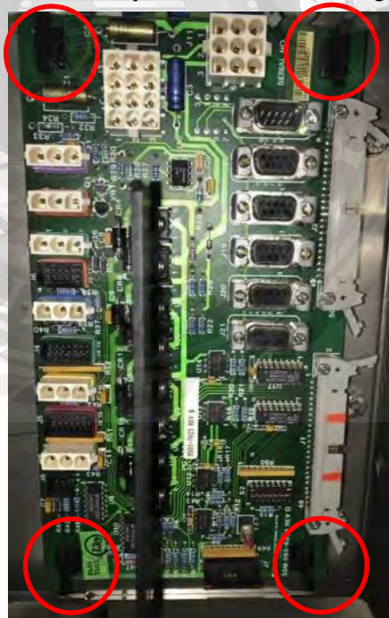
Figure 5-5 Unlatch Latches on the IFM Board
