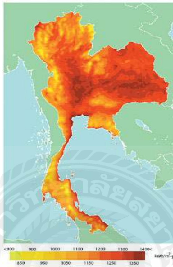
Figure 5 Areas with solar power potential
