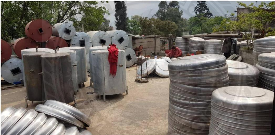
FIGURE 3.6 Water tanks being cleaned for finishing.
