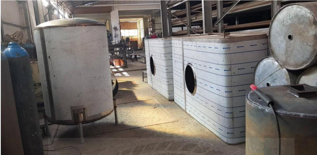
FIGURE 3.5 Special water tanks being produced
