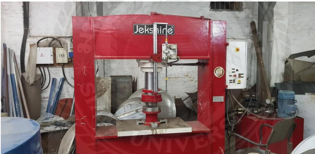
**FIGURE 3.9** A press machine used to shape the water tanks.
