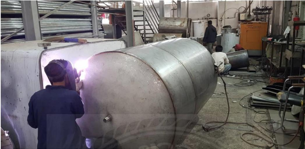
**FIGURE 3.8** Water tank being welded.
