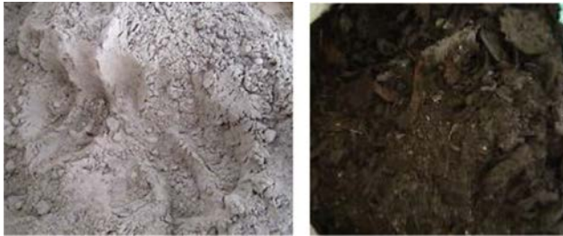
Fig. 1. Show physical of fly ash powder, Mae Moh, Lampang Province and banana peel charcoal powder
