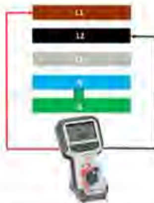
Figure 1 Show connections for insulation resistance test of LV Switchgear
