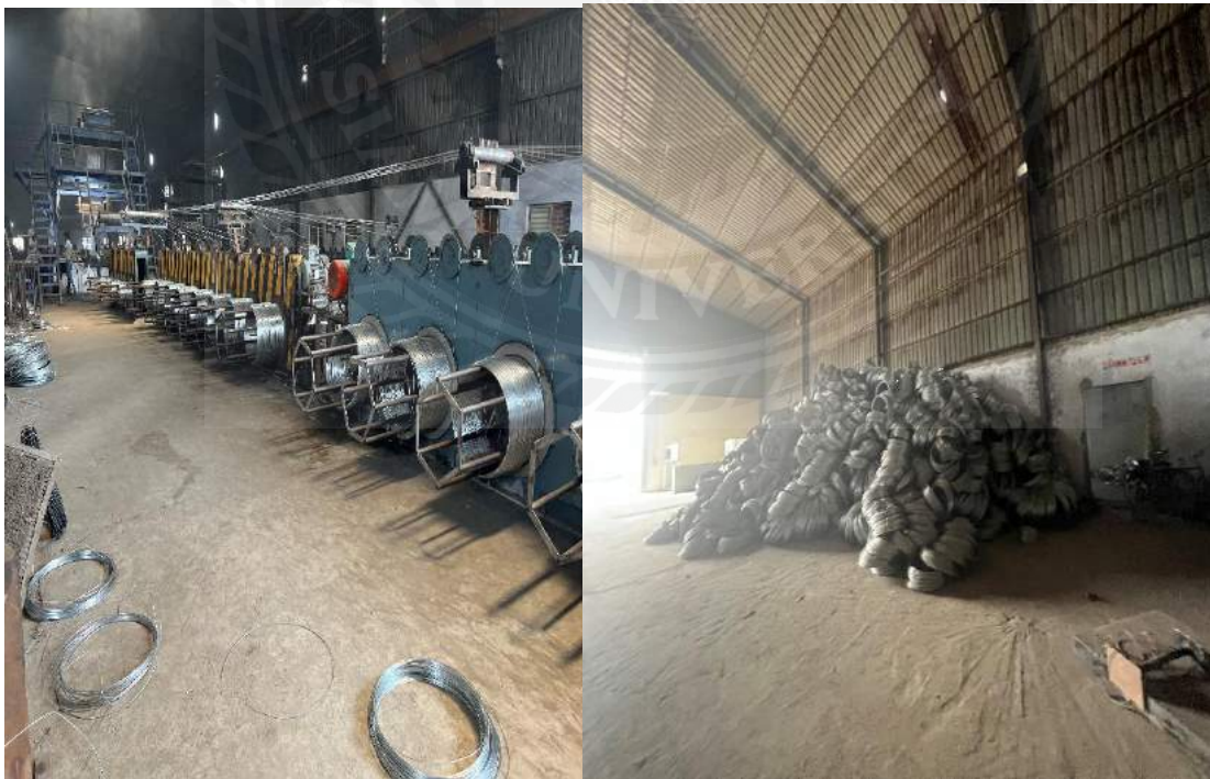
Figure 8: G.I wire machine and final product.
