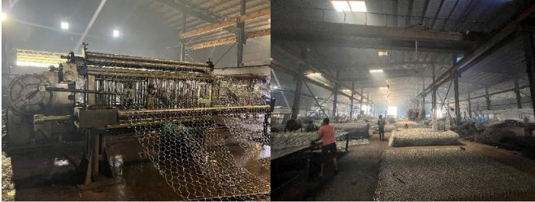
Figure 9: Gabion machine production and preparation.
