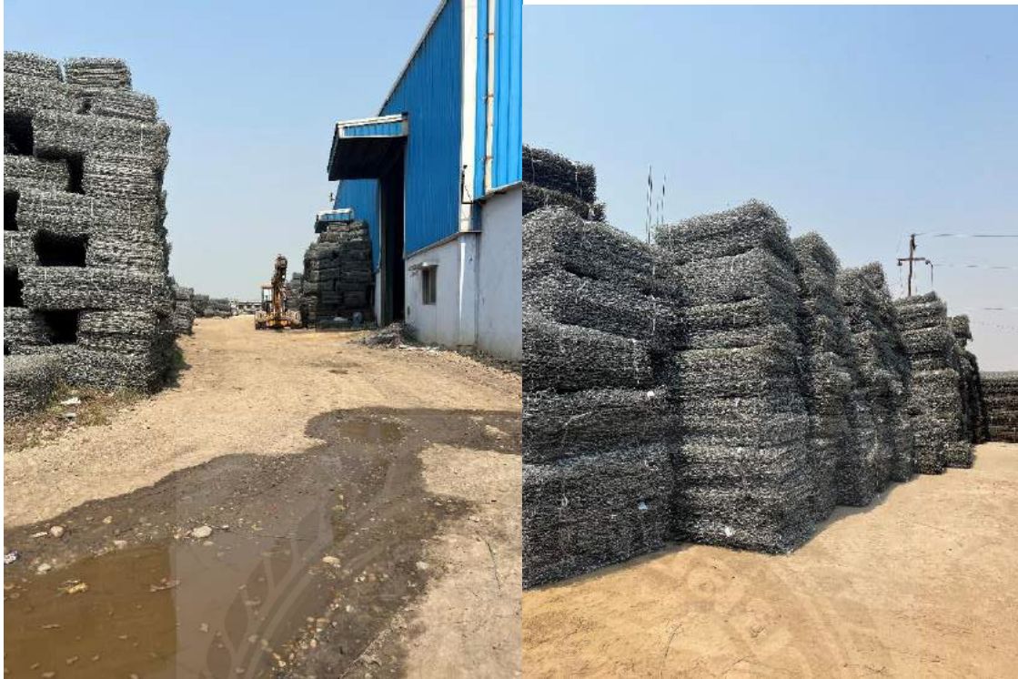
Figure 5: Gabion box in stock
