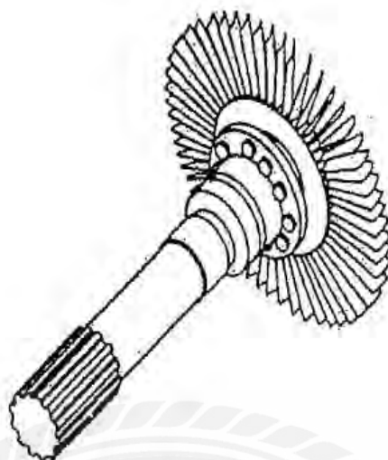
FIGURE 1-51. Rotor element of the turbine assembly.
