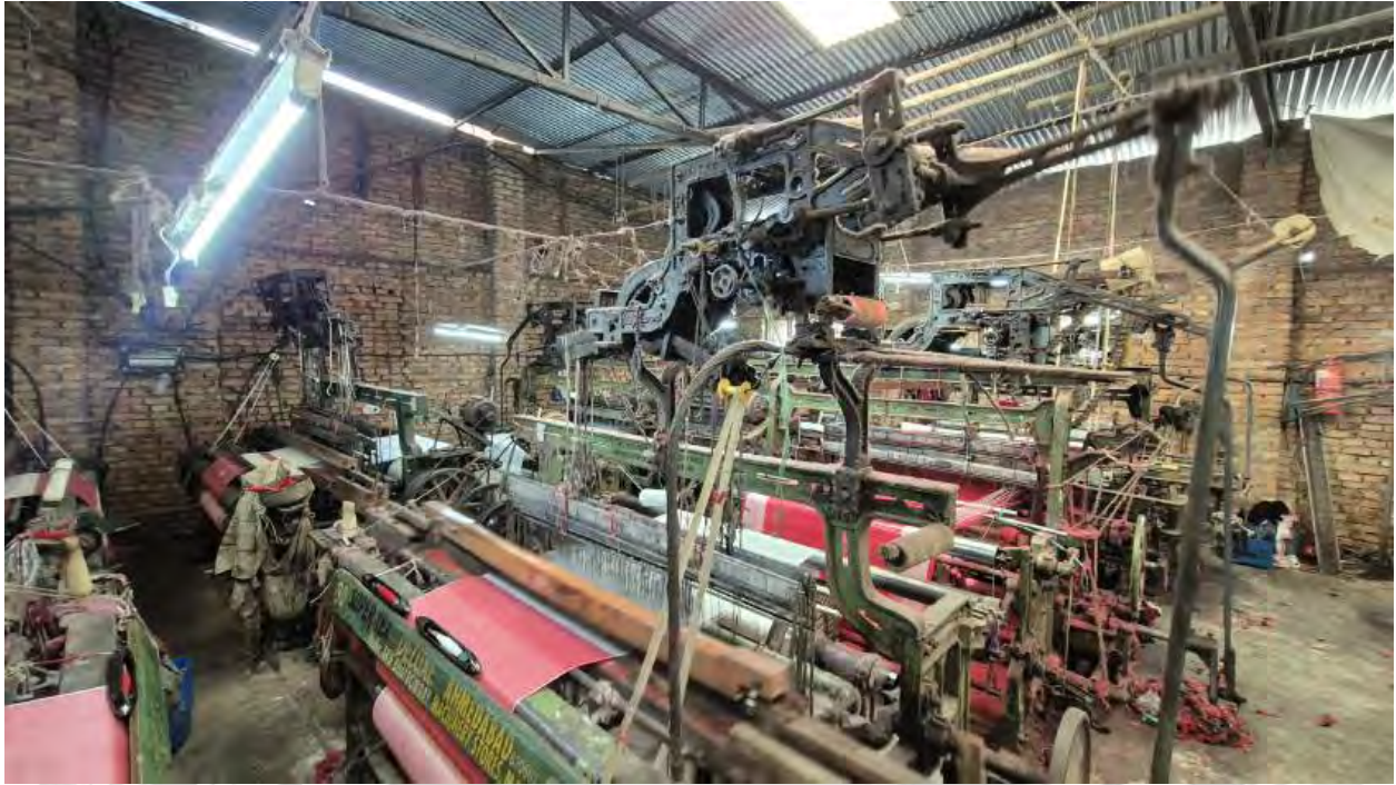
Figure 13: Power Looms with Dobby System Integrated
