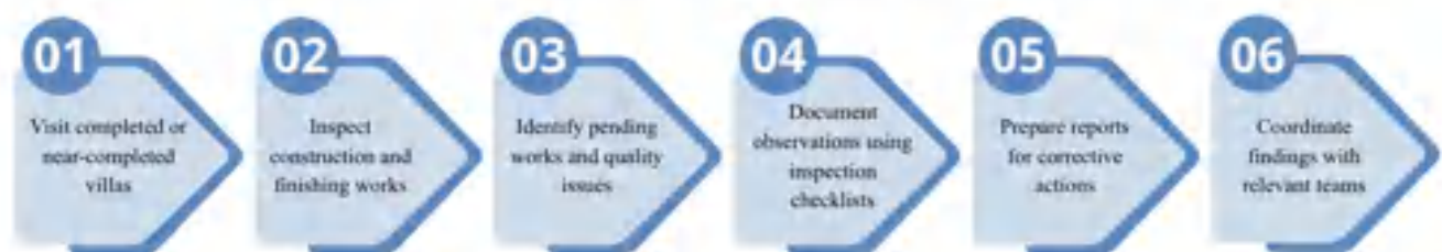
Figure 14: Job Process for Pre-Handover Inspection and Quality Assessment
